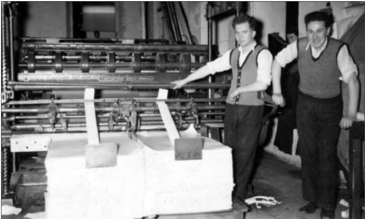
Sam Crofton and John Gray at the West End Cutter. This Cutter cut all the paper from number two machine. The paper being cut on this Cutter had to be cut to register, which meant that if the sheet was supposed to have four water marks we'll say such as Swiftbrook Bond in each sheet. The mark was able to move up and down in the sheet and it had to be kept centred and that was the job to keep an eye on that and if it was going off centre there was a wheel on the side of the machine and you just adjusted that to get the water mark square.
