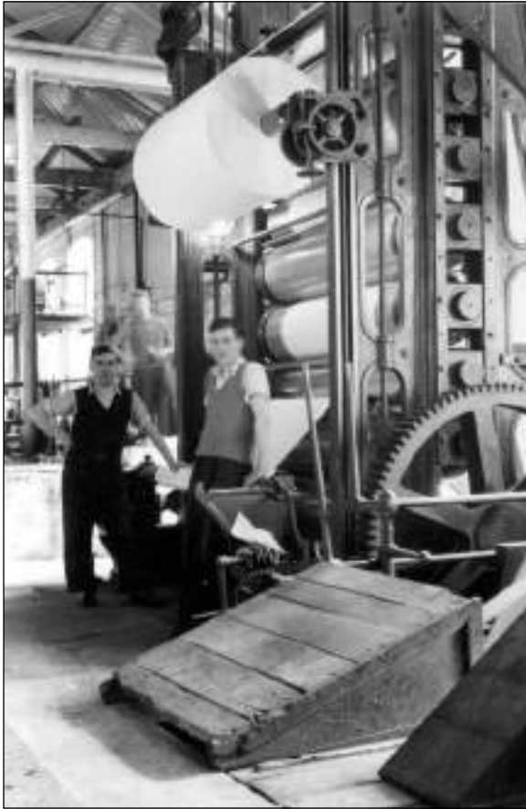
This is number one calender with Tony McDermott and Jim Grace standing at the reel. These calenders were used to put the glaze on the paper. There were steel rolls and the two big rolls that you can see behind Jim's head there were rolls made of a very hard cotton. They put the glaze on the paper. The degree of glaze was achieved by levers at the back of the back of the calender. Weights were put on or taken off to suit the glaze that was required.
