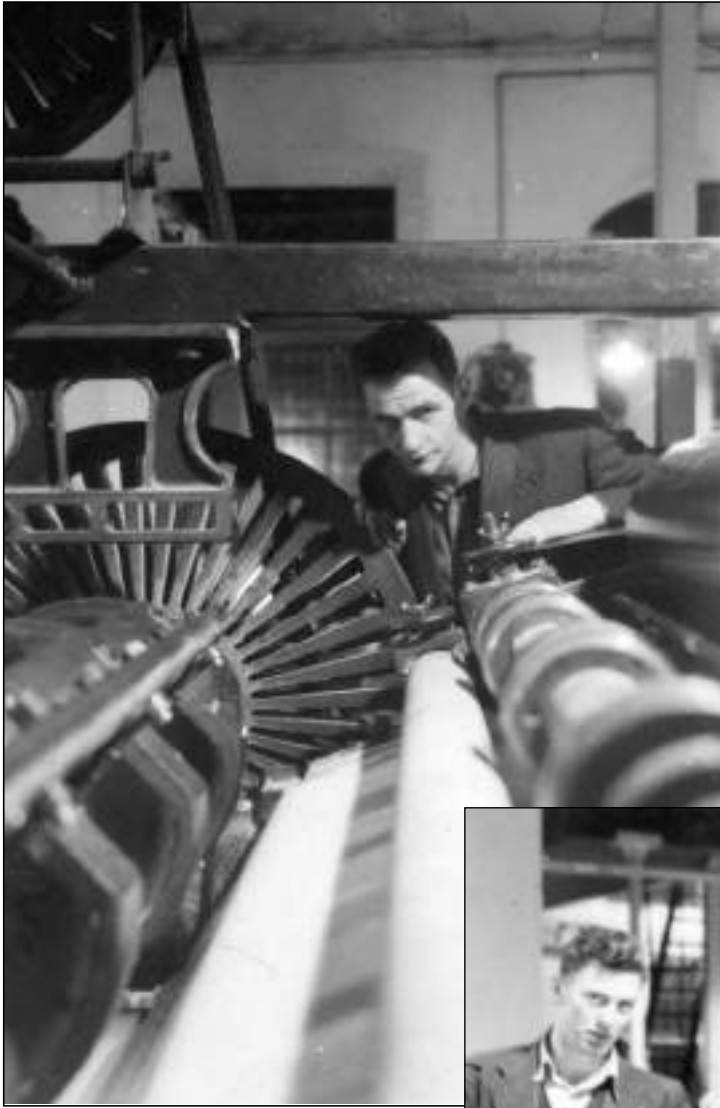
Kit Brady at number one cutter with the circular knives across on the right and the chopping blade on the left. The circular knives cut the sheet lengthwise and the chopper cut them off to the length that was required.
