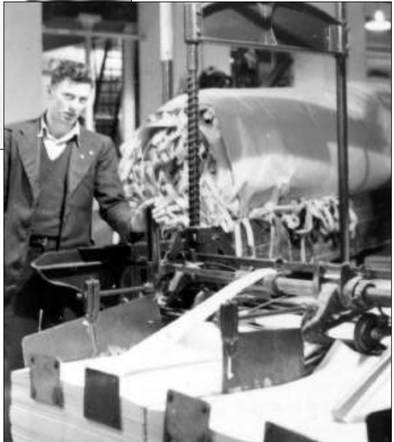
Another view of number one cutter with Willie McEntee. The roll of shavings at the back are shavings from the Cutter. They have to be brought back up to the beating loft and reused.
