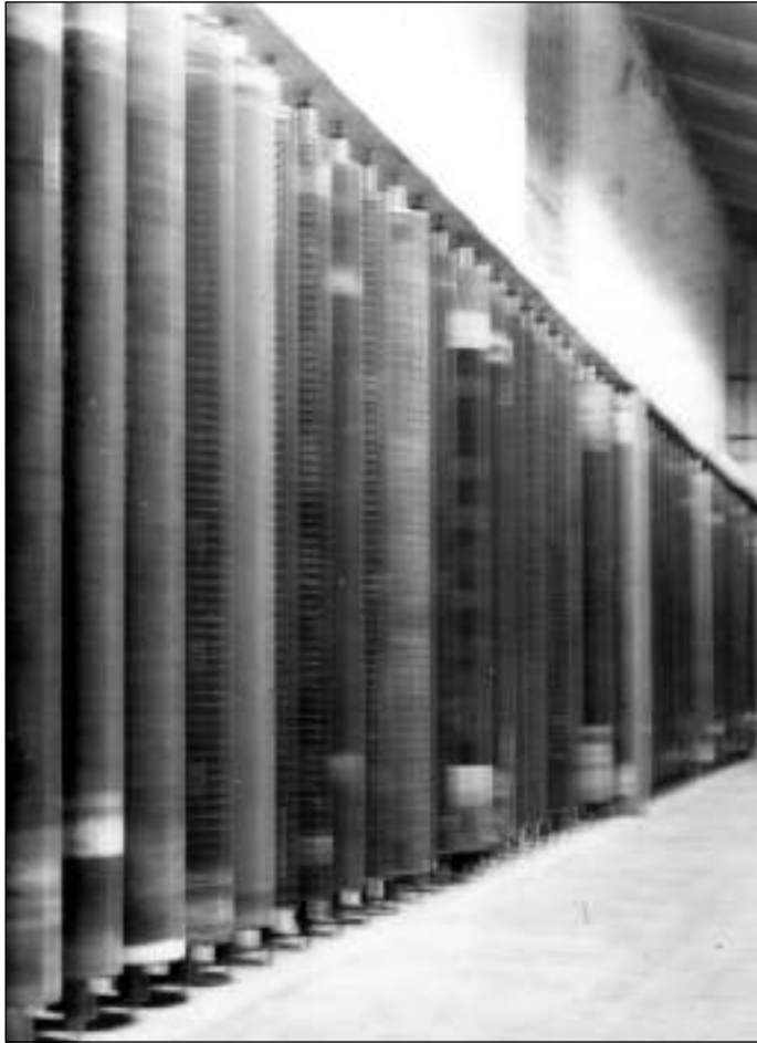
A view of the dandy room. This is the room where the dandies were kept. The dandies were the instruments used to put the watermark in the paper. There was one dandy there with the name of the previous owner of the mill, McDonnell, on it. This family owned the mill before Mr. Horsborough and his company took it over. The family died out and it was left to the last surviving member, a Jesuit priest. As he could not take over the mill, it had to be sold.
