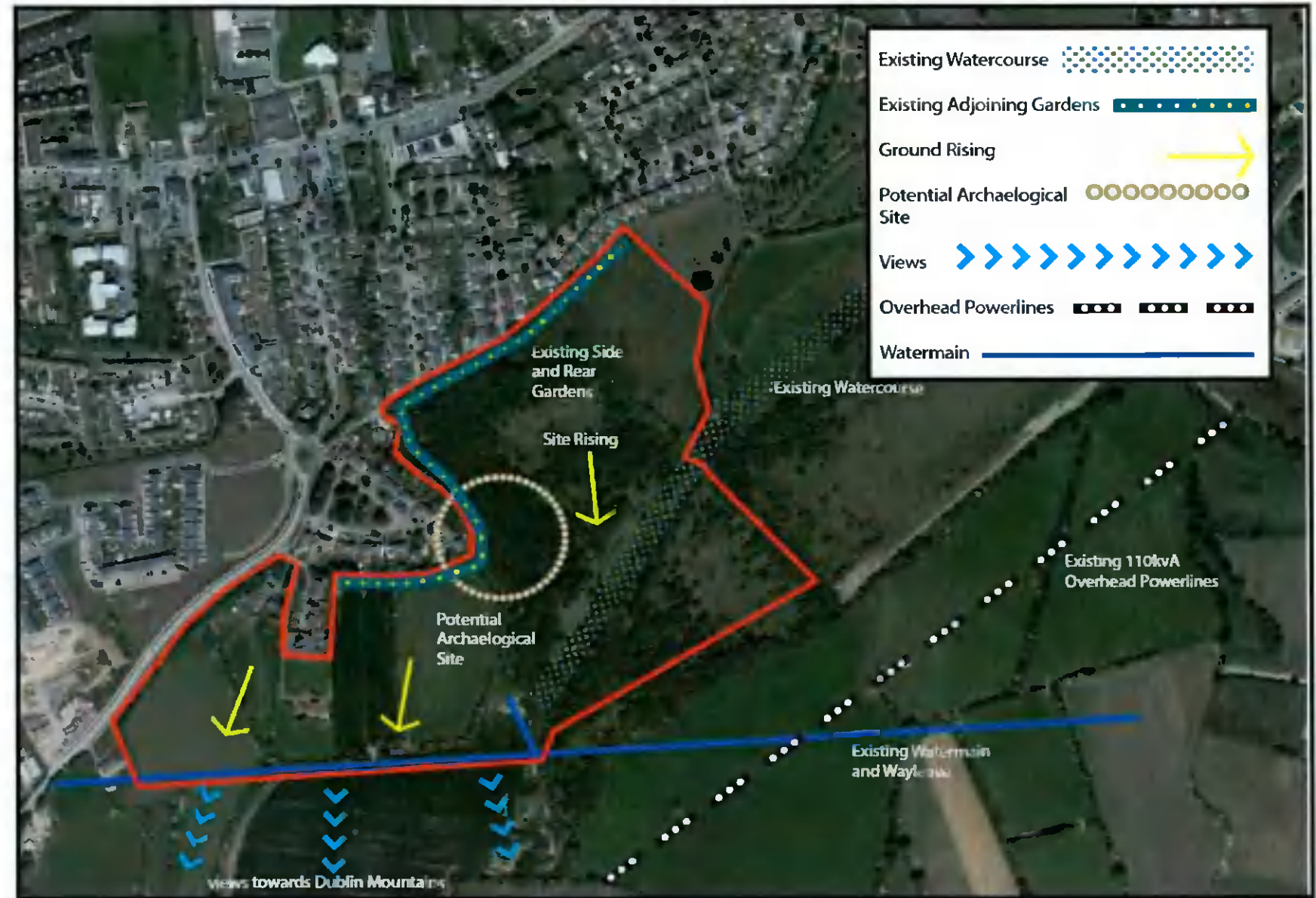
Figure 4.2: Site Constraints Source: C&W O'Brien Architects
